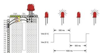
We can use the onboard power and the breadboard to attach some LED lights, and write a program to control when they turn on and off. Once we know how to turn them on/off, we can decide why we might want to flash the lights, and then incorporate that into solving a bigger problem.
