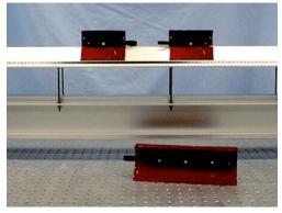
Separate the photogates on the air track to create a collision interval. The first cart should be placed before the first gate, and the second cart should be placed in the collision interval between the gates. Make sure that the air blower is running before you slide the cart on the track. Sliding the cart when the blower is off will damage the track.
