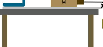
When the system is released from rest, the cart should experience constant acceleration as it moves down the track. This acceleration and the measured tension will be used to determine the coefficient of friction.
