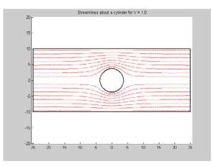
Fig. 6 Streamlines about a cylinder for V = 1.0
