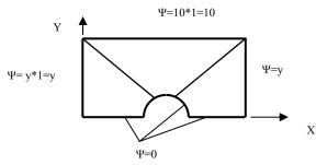
Fig.5 Boundary conditions for stream function
