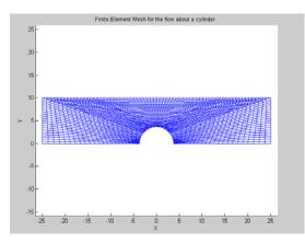
Fig. 4 Finite element mesh for the flow about a cylinder (2376 elements and 2507 nodes)
