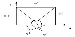
Fig. 7 Boundary conditions for temperature field
