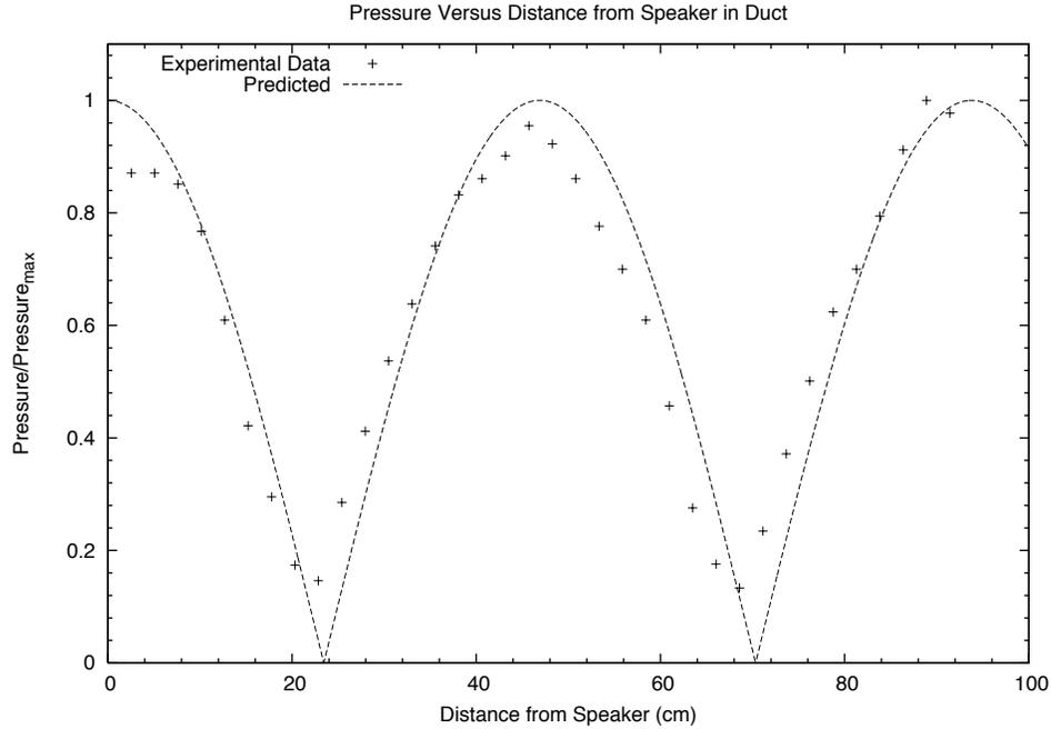
Figure 7: The horizontal difference between the experimental data and the predicted pressure curve may arise from the fact that 0 cm corresponded to the speaker’s mount and not to the location at which the speaker was emitting maximum pressure.
