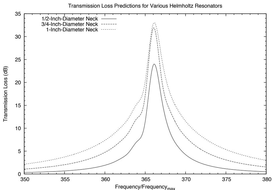
Figure 4: The transmission loss predictions for three Helmholtz resonators of varying size. The dimensions of each resonator is outlined in Table 3. The 'bump' located on the left of the three resonance curves is probably a result of the Mathematica program not iterating in small enough increments.
