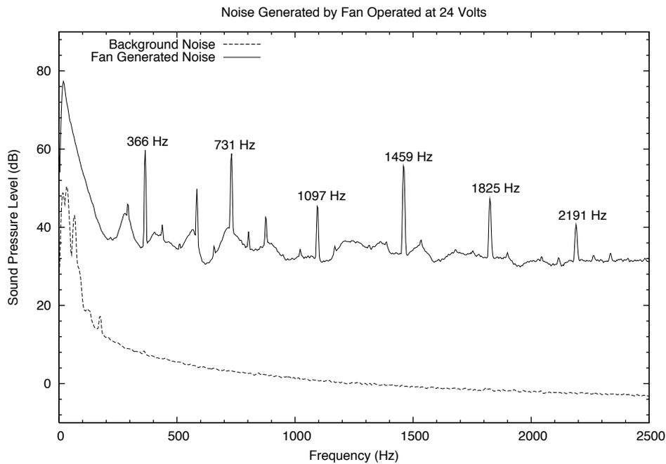
Figure 9: The harmonic frequencies of the fan are labeled with their respective frequencies. The frequency resolution for this average is approximately 3 Hz.
