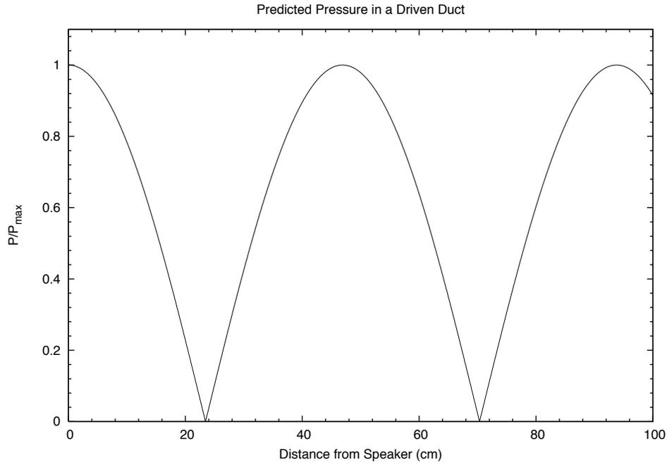
Figure 3: At  $x=0$  (the theoretical position of the speaker), there exists a pressure maximum. For a 366 Hz tone, the next pressure maximum is located half a wavelength away or approximately 46.86 cm.
