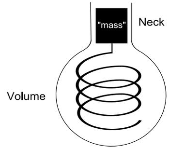
Figure 1: Motion of air within a Helmholtz resonator.
