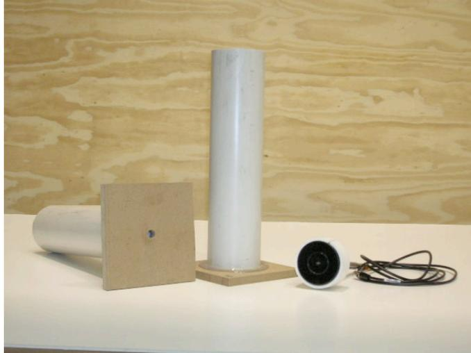
Figure 10: The two Helmholtz resonators pictured here have neck diameters of  $\frac{1}{2}$  in and  $\frac{3}{4}$  in. The plunger on the far right was equipped with a Brüel & Kjaer Type 4138  $\frac{1}{4}$ -in microphone that served as a tool for accurate tuning of the resonator.
