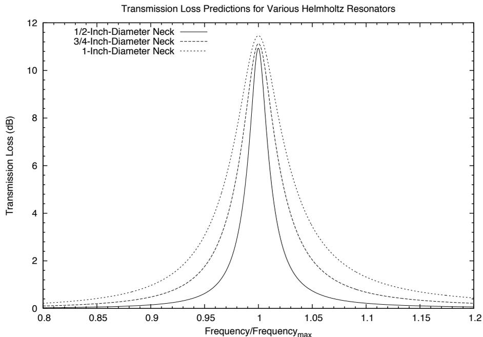
Figure 5: The transmission loss predictions using Equation 13, which accounted for grazing flow with a negligible Mach number. Note that the x-axis shows the frequency divided by the frequency at which there is maximum transmission loss. Because the resonance frequencies for each Helmholtz resonators were not equal to one another, this x-axis allowed the predictions to be aligned so that the effects of the resonators could be compared.
