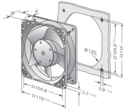
(b) Dimensions of the fan in mm.[8]
