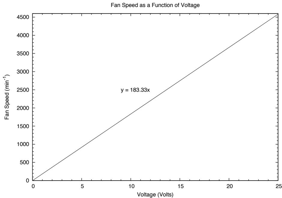
Figure 16: Assuming that the fan speed is linearly proportional to the voltage supplied to the fan, it is possible to use known information from the fan's specifications sheet to determine the proportionality constant. Multiplying the voltage by this constant should yield an approximation to the fan's speed.
