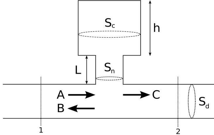
Figure 2: A cylindrical Helmholtz resonator attached to a duct as a side-branch. The dimensions of the Helmholtz resonator include a volume of cross-sectional area  $S_{cavity}$ , height  $h$ , neck of cross-sectional area  $S_{neck}$ , and length  $L$ . The duct has a cross-sectional area of  $S_{duct}$ .  $A$  represents the acoustic wave originating from a source, and  $B$  and  $C$  are the reflected and transmitted waves, respectively.
