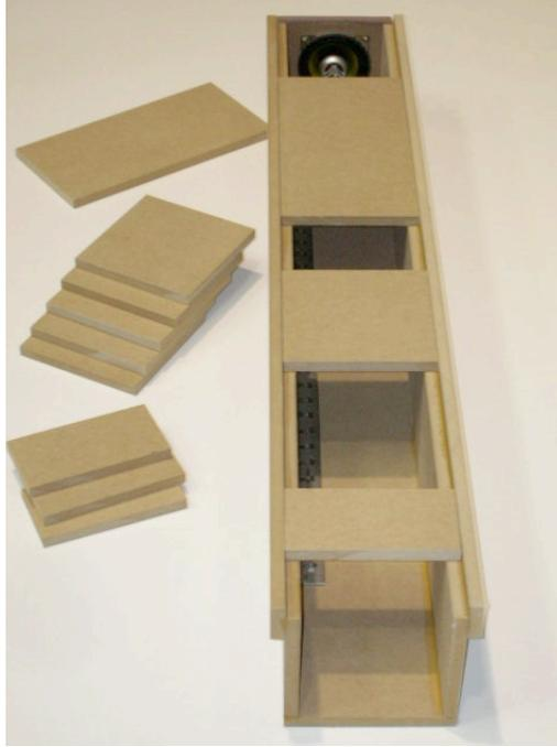
Figure 6: The experimental duct shown with its multiple, moveable lids. This picture shows the duct set up for measuring the pressure within the duct. A yardstick placed at the bottom of the duct allowed for accurate placement of the microphone used to make pressure measurements within the duct. The speaker mounted at the end of the duct served as the pressure source during this measurement. The speaker and its mount could be removed, allowing for the placement of a fan.
