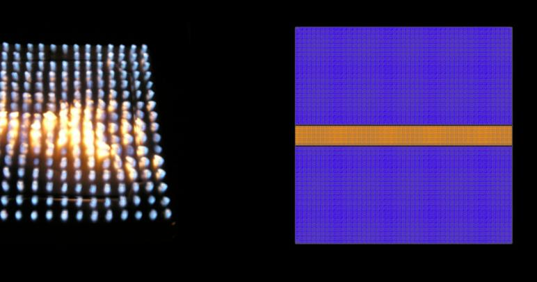
m = 0, n = 1  $f_{obs} = 705$  Hz  $f_{exp} = 641$  Hz  $%_{rel error} = 10$
