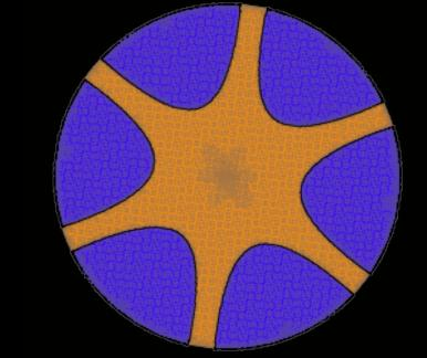
m = 3, n = 1  $f_{obs} = 1740$  Hz  $f_{exp} = 1713$  Hz  $%_{rel error} = 1.6$
