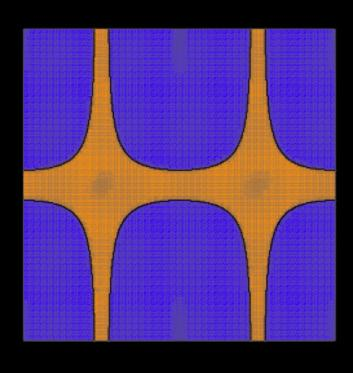
m = 2, n = 1  $f_{obs} = 1500$  Hz  $f_{exp} = 1433$  Hz  $%_{rel error} = 4.7$
