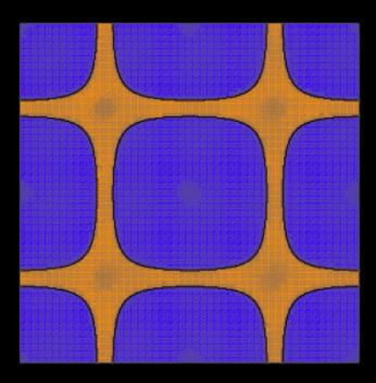
m = 2, n = 2  $f_{obs} = 1880$  Hz  $f_{exp} = 1812$  Hz  $%_{rel error} = 3.8$
