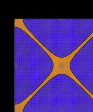
m = 2, n = 0 $f_{obs} = 1320 \text{ Hz} f_{exp} = 1281 \text{ Hz} \$_{rel error} = 3.0$
