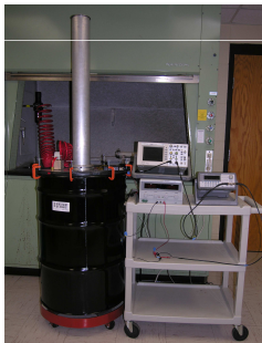
Helmholtz Resonator System with 1.0m Neck Installed
