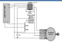
A LM 335 was used to construct a temperature sensor for the system. The HOBOware U12-006 data logger can only measure voltages ranging from 0 to 2.5V. The voltage measured from the LM 335 was higher than this, so a voltage divider was used to lower the signal form the temperature sensor. A pressure sensor was used to measure a change in air pressure. The signal received from
