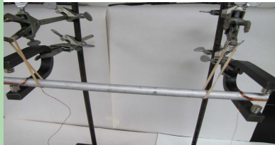
Figure 1: In this figure, the aluminum bar was used as an example to show how the apparatus was set such that a free-free boundary was used.
