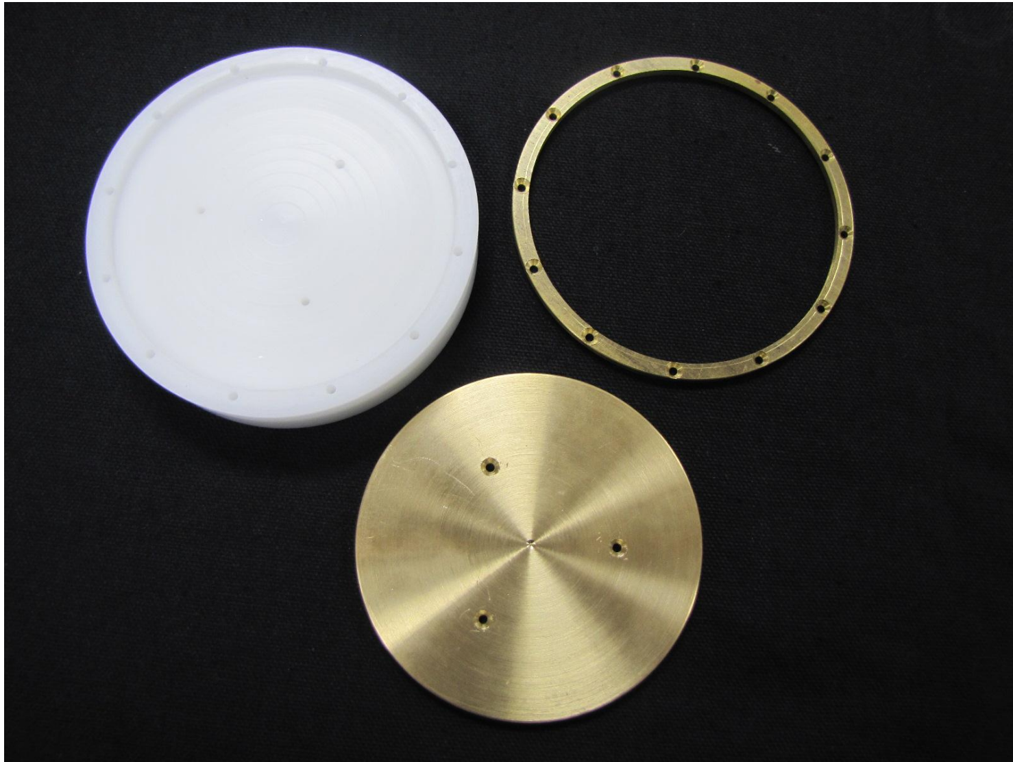
Figure 3: Disassembled transducer. Clockwise from left: Delrin plastic base, brass tensioning ring, brass backing plate.
