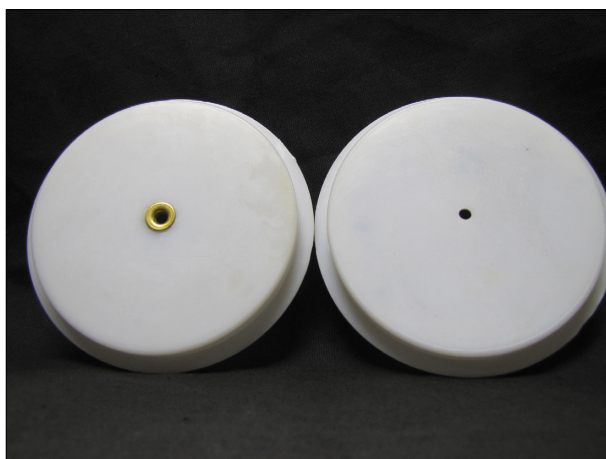
Fig. 3. PVC test caps with holes drilled in the center, grommet and no grommet case shown.
