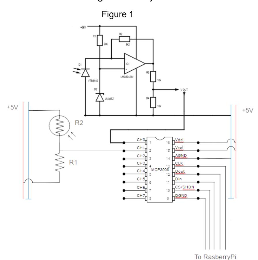
The python code function, readADC\_channel\_0 in Figure 4 gives the Rasberry Pi the ability to convert the analog input to a digital input. The MCP3008 chip is a 10-bit chip
