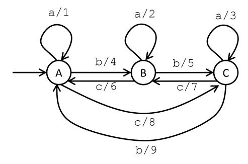
1) Given the finite state machine illustrated below, find the output for the input string "abc"
