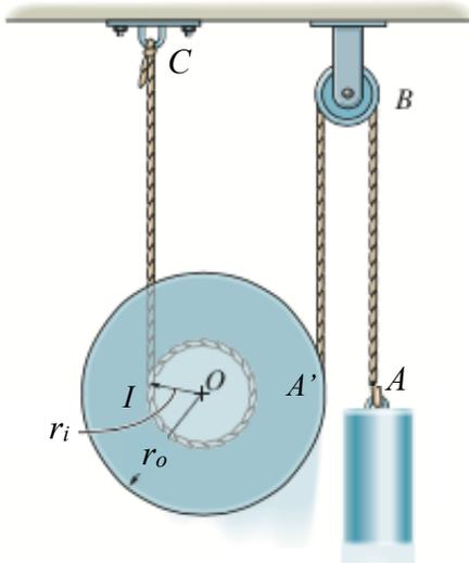
The spool has an inner radius  $r_i = 0.25\text{m}$ , and an outer radius  $r_o = 0.5\text{m}$ . It has a mass  $m_o = 15\text{ kg}$  and its radius of gyration  $k_o = 0.35\text{m}$ . A cylinder with mass  $m_A = 20\text{ kg}$  is attached to the cord at A, then released from rest. Determine the tensions  $T_A$  and  $T_C$  in the two cords, and angular velocity  $\omega$  of the spool at  $t = 3\text{ s}$ . Neglect the masses of the pulley and cord.
