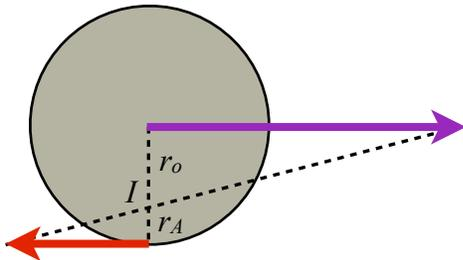
The center O of the gear and the gear rack P move with the B velocities and accelerations shown. Determine the angular acceleration  $\alpha$  of the gear and the vector acceleration  $\mathbf{a}_B$  of point B located at the rim of the gear at the instant shown.
