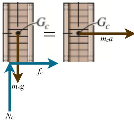
$$\begin{aligned} \Sigma F_x &= f_c = m_c a \\ \Sigma F_y &= N_c - m_c g = 0 \end{aligned}$$
