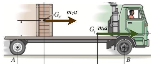
$$\begin{aligned} \Sigma F_x &= f_A = (m_c + m_t) a \\ \Sigma F_y &= N_A + N_B - (m_c + m_t) g = 0 \\ (\curvearrowright +) \Sigma M_A &= (m_t g) x_{At} + (m_c g) x_{Ac} - (N_B) x_{AB} = (m_t a) y_{At} + (m_c a) y_{Ac} \end{aligned}$$
