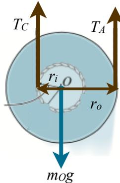
$$\begin{aligned} m_o v_{oi} + (\Sigma F) t &= m_o v_o \\ 0 + (T_A + T_C - m_o g) t &= m_o v_o \\ (T_A + T_C - m_o g) t &= m_o (\omega r_i) \\ T_A(3) + T_C(3) - (15)(9.8)(3) &= (15)(0.25)\omega \\ 3T_A + 3T_C - 3.75\omega &= 441 \end{aligned}$$
