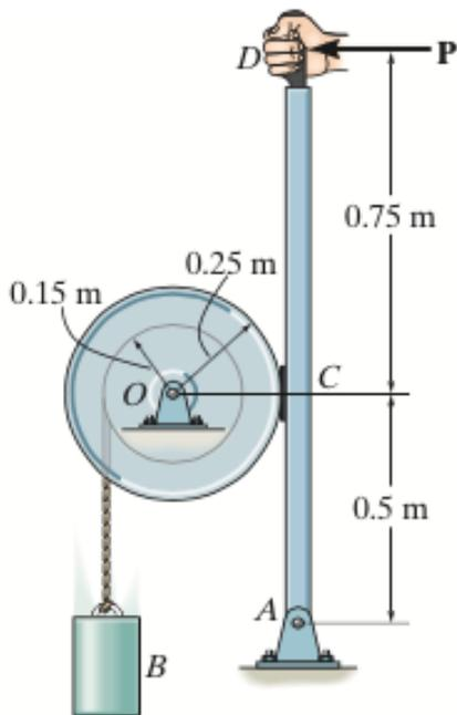
The drum has a mass  $m_o = 40$  kg and a radius of gyration about the pin at O of  $k_o = 0.20$  m. The suspended block B has a mass  $m_B = 10$  kg. It is released from rest and allowed to fall 2.5 m *without applying the brake ACD*. Determine the speed  $v_B$  of the block at this instant.
