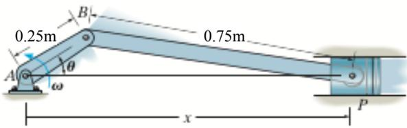
The crankshaft AB is rotating at a constant angular velocity of  $\omega_{AB} = 125$  rad/s. Determine the velocity of the piston  $v_P$  at the instant  $\theta = 30^\circ$ .
