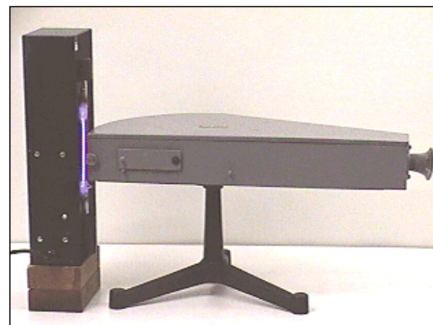
If you are not seeing lines, have your instructor check that the spectroscope is in alignment with the lamp.
