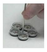
A long straight ire is surrounded by a ring of small magnetic compasses, as demonstrated in lab. A current passes through the wire.
