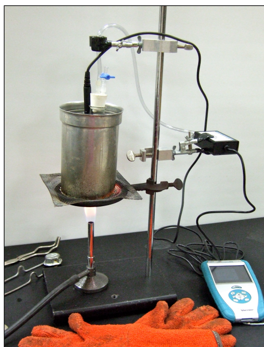
Make sure the blue release valve on the stopper is closed before you begin data collection.
