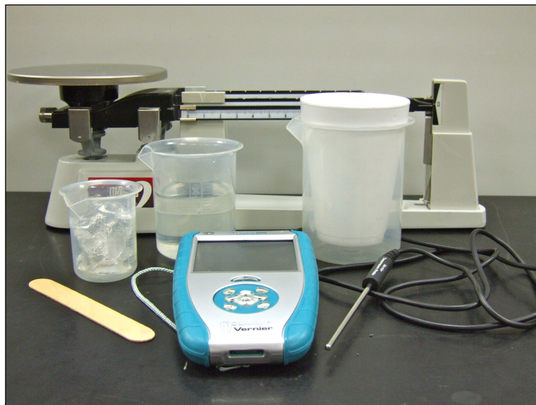
Use the tongue depressor to get the ice into the styrofoam calorimeter cup without splashing.
