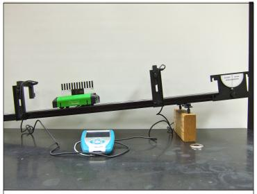
Make sure that photogates are triggered by the wide blockout gap on the fence, and not the small pickets!
