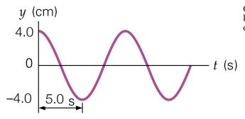
On the left is a graph illustrating the vertical oscillation of a 1 kg mass attached to a spring. Assume that up is the positive direction, and down is the negative direction.
