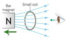
We want to use the magnet shown on the left to induce a current in the closed loop of wire. As shown in the picture, your eye is at some position +x, and you are looking at the loop in the yz-plane. The magnet is pulled away from you, in the -x direction.
