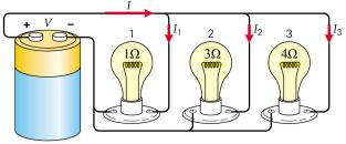
The same three bulbs on the right are now wired in parallel to the 24V battery as shown.
